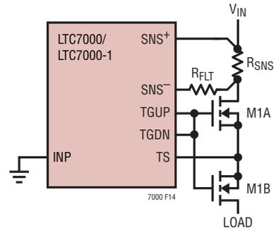
Figure 14. Protecting Load from Voltage Drops on  $V_{IN}$
