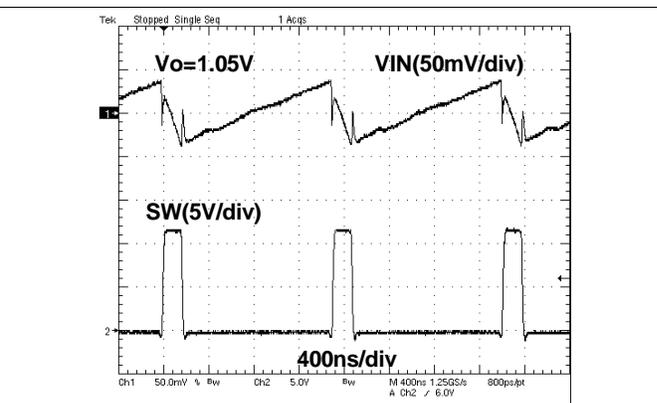
Figure 15. Voltage Ripple at Input
