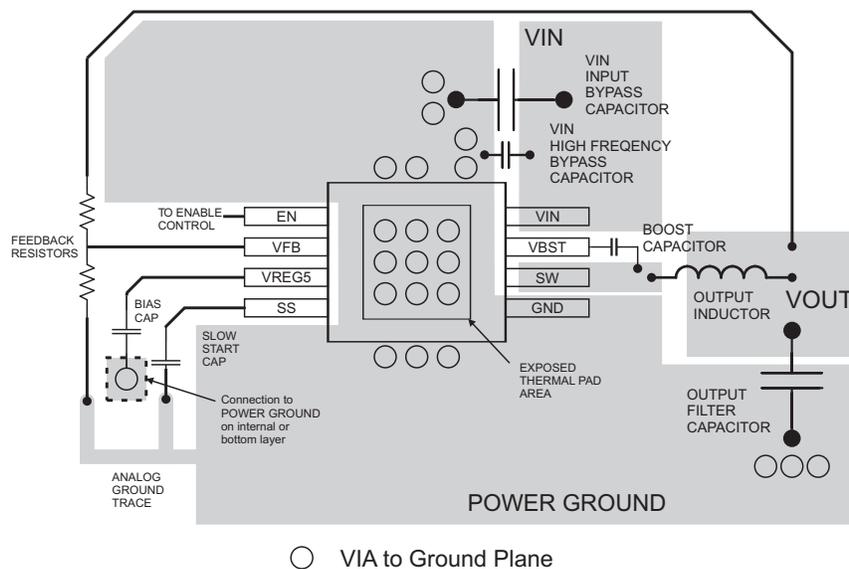
**Figure 16. PCB Layout**
