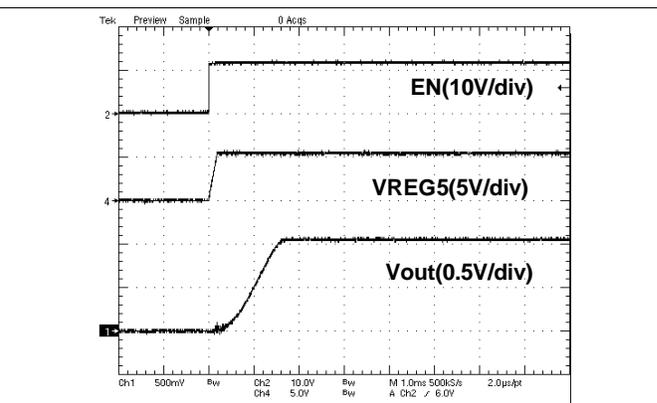
Figure 13. Start-Up Waveform
