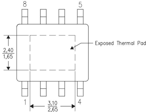
**Figure 17. Thermal Pad Dimensions**
