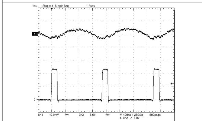
Figure 14. Voltage Ripple at Output
