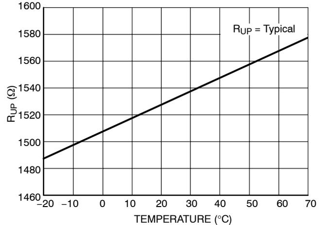
Figure 4. R<sub>UP</sub> vs. Temperature
