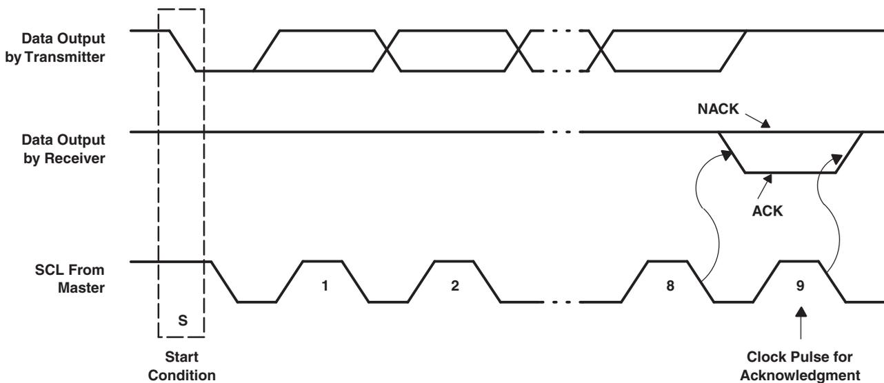
**Figure 13. Acknowledge on I<sup>2</sup>C Bus**
