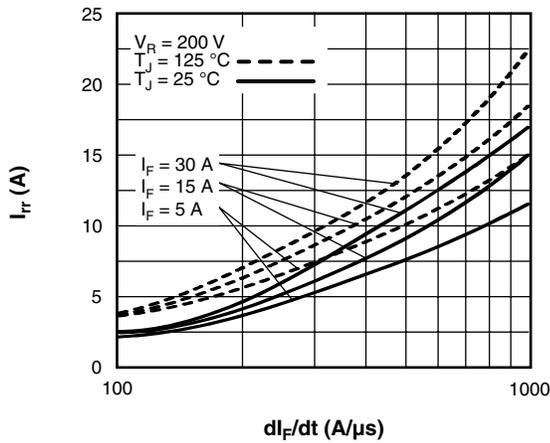
Fig. 6 - Typical Recovery Current vs.  $di_F/dt$
