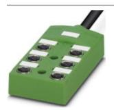
Sensor/actuator box, application: Standard, connection method: M12-SPEEDCON-socket Metal, number of slots: 6, number of positions: 5, coding: A - standard, slot assignment: Double, status display: No, Universal; master cable connection: Fixed connection 180°, PUR/PVC, cable length: 5 m, shielding: no
