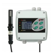
Humidistat, thermostat with two relay outputs. T+RH probe from hard anodized duralumin for compressed air up to 25 bars with 1 meter cable. Outdoor, indoor use.
