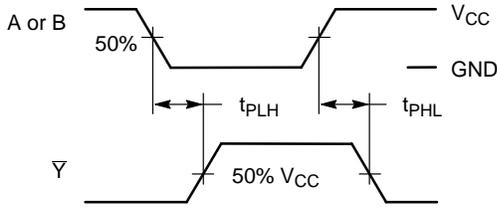
Figure 3. Switching Waveforms
