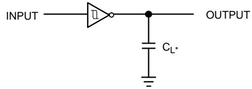
\*Includes all probe and jig capacitance.
