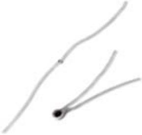
111 Series, small glass bead with axial leads, 2,000 Ohm resistance,  $\pm 25.0\%$  tolerance, 25/85 BETA = 3068
