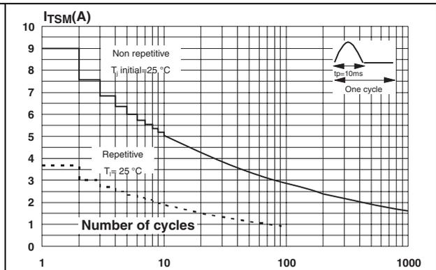
Figure 11. Non repetitive surge peak on state current for a sinusoidal pulse and corresponding value of  $I^2t$
