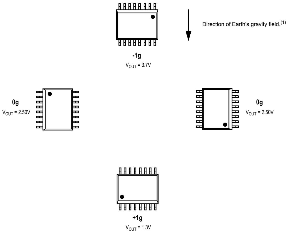
1. When positioned as shown, the Earth's gravity will result in a positive 1g output
