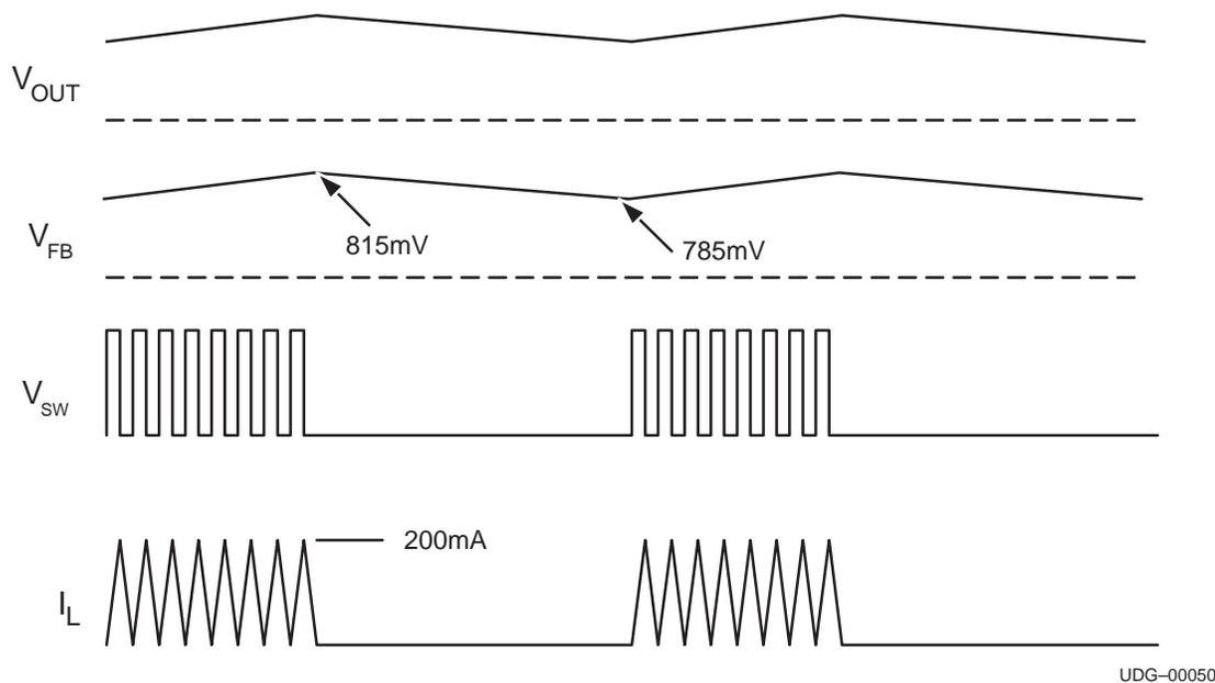
Figure 4. Typical Pulsed-Variable-Frequency Mode (PFM) Circuit Waveform
