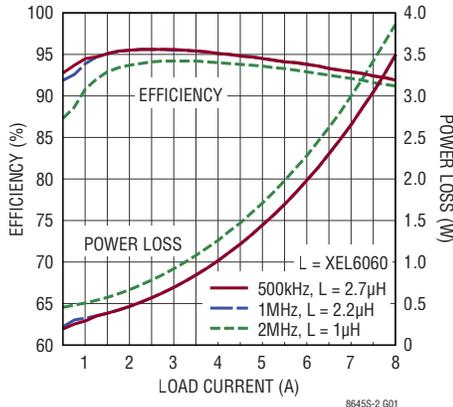
**12V<sub>IN</sub> to 3.3V<sub>OUT</sub> Efficiency vs Frequency**
