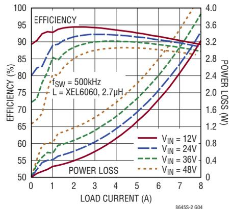
**Low Load Efficiency at 5V<sub>OUT</sub>**
