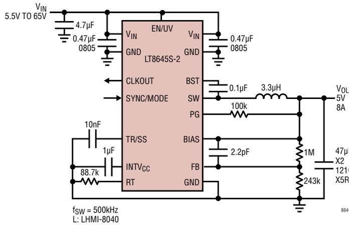
**3.3V, 8A Step-Down Converter with Soft Start and Power Good**
