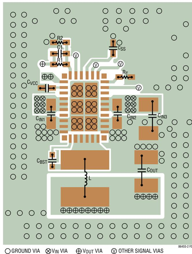
Figure 1. Recommended PCB Layout for the LT8645S-2
