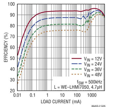
**Low Load Efficiency at 3.3V<sub>OUT</sub>**
