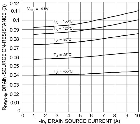
Figure 18 Typical On-Resistance vs. Drain Current and Temperature
