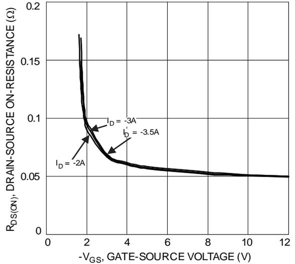
Figure 17 Typical Drain-Source On-Resistance vs. Gate-Source Voltage
