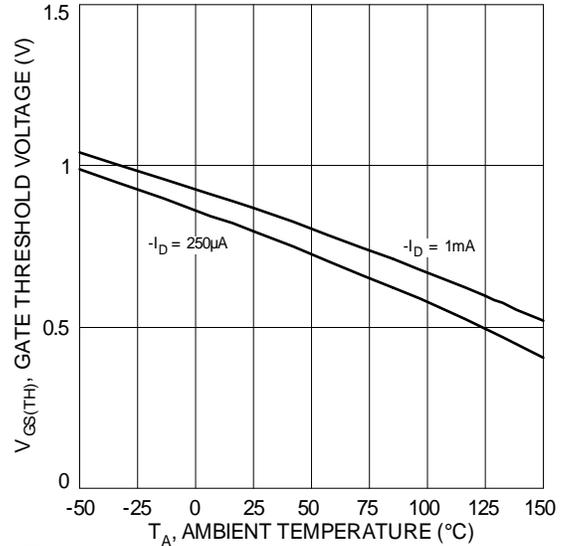
Figure 21 Gate Threshold Variation vs. Ambient Temperature
