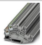
Multi-level terminal block, Cross section: 0.14 mm² - 1.5 mm², AWG: 26 - 14, Connection type: Push-in connection, Width: 3.5 mm, Color: gray, Mounting type: NS 35/7,5, NS 35/15
