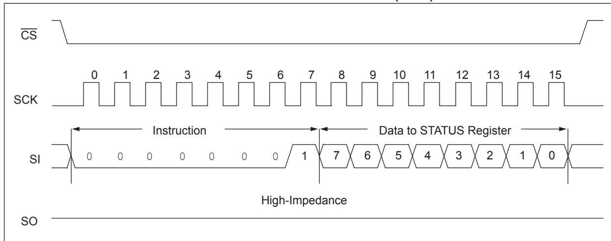
**Note:** An internal write cycle ( $T_{wc}$ ) is initiated on the rising edge of  $\overline{CS}$  after a valid write STATUS register sequence.
