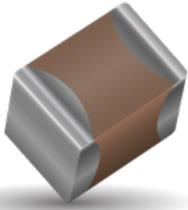
X7R formulations are called “temperature stable” ceramics and fall into EIA Class II materials. X7R is the most popular of these intermediate dielectric constant materials. Its temperature variation of capacitance is within  $\pm 15\%$  from  $-55^{\circ}\text{C}$  to  $+125^{\circ}\text{C}$ . This capacitance change is non-linear.
