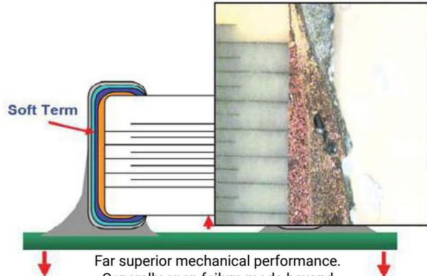
Far superior mechanical performance. Generally open failure mode beyond 5mm flexure
