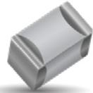
KYOCERA AVX has developed a range of multilayer ceramic capacitors designed for use in applications up to 150°C. These capacitors are manufactured with an X8R and an X8L dielectric material. X8R material has capacitance variation of ± 15% between -55°C and +150°C. The X8L material has capacitance variation of ±15% between -55°C to 125°C to 125°C and +15/40% from +125°C to +150°C.
