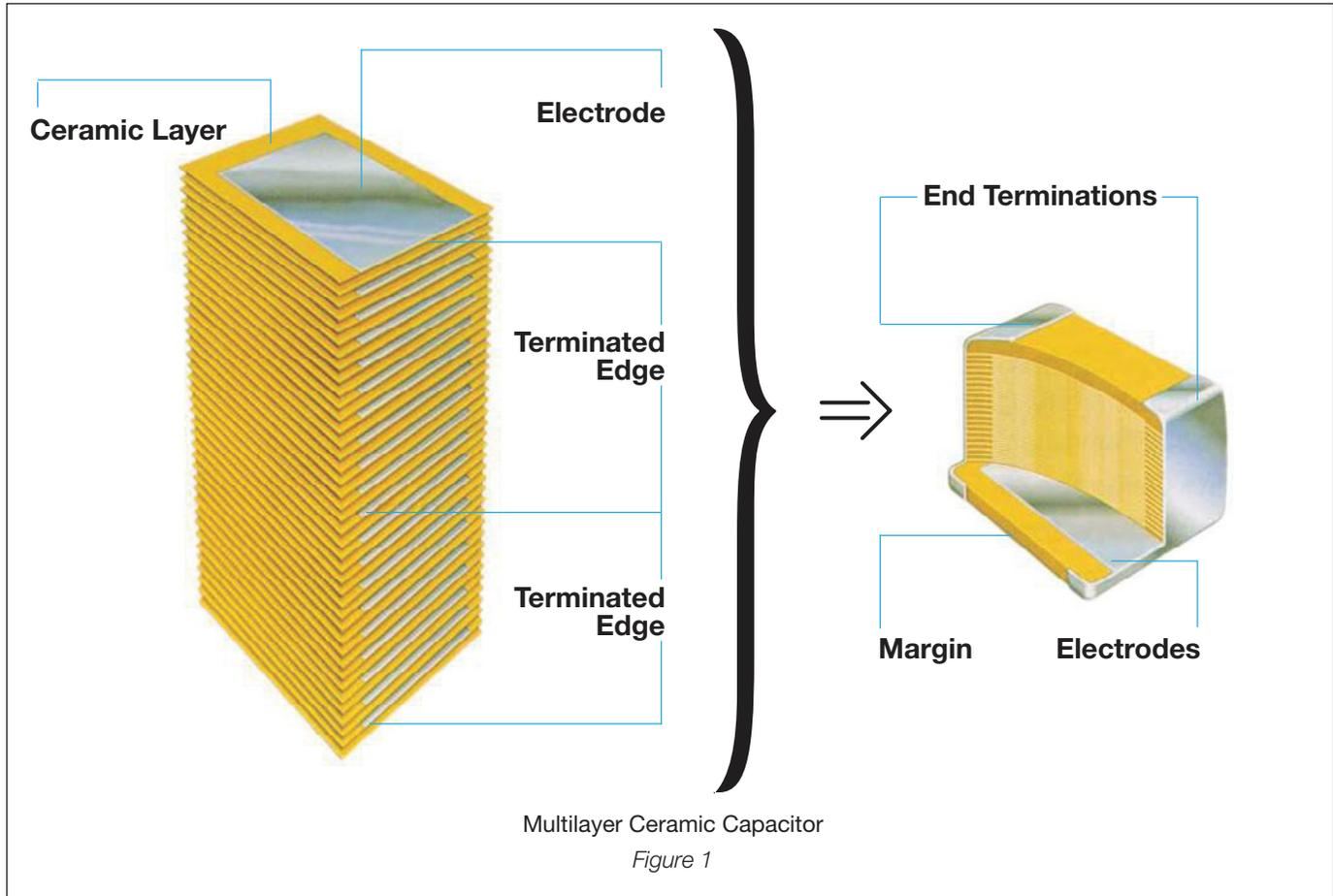
**Formulations** – Multilayer ceramic capacitors are available in both Class 1 and Class 2 formulations. Temperature compensating formulations are Class 1 and temperature stable and general application formulations are classified as Class 2.
