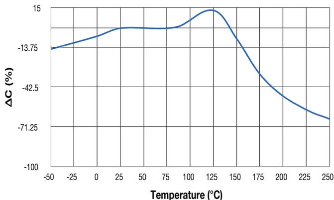
Typical Temperature Coefficient of Capacitance (COG Dielectric)
