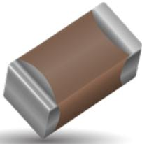
High value, low leakage and small size are difficult parameters to obtain in capacitors for high voltage systems. KYOCERA AVX special high voltage MLC chips capacitors meet these performance characteristics and are designed for applications such as snubbers in high frequency power converters, resonators in SMPS, and high voltage coupling/DC blocking. These high voltage chip designs exhibit low ESRs at high frequencies.
