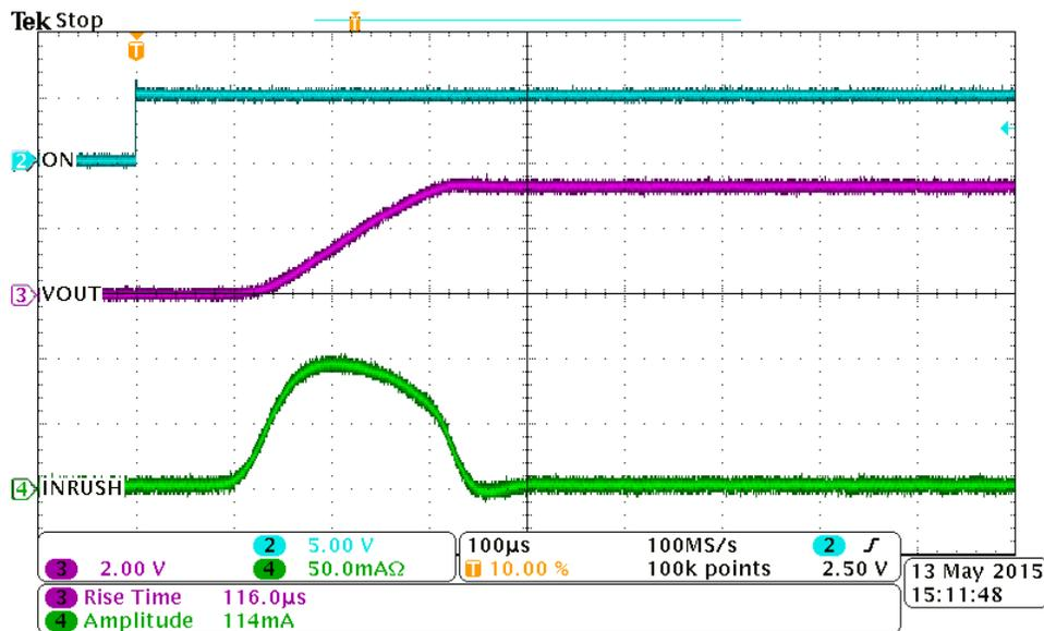
Figure 40. TPS22932B Inrush Current With 4.7-µF Output Capacitor
