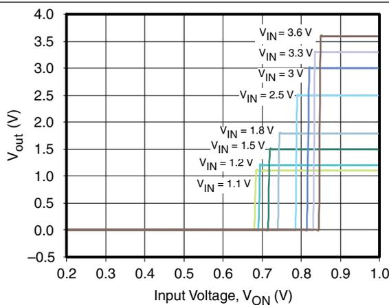
Figure 10. ON-Input Threshold
