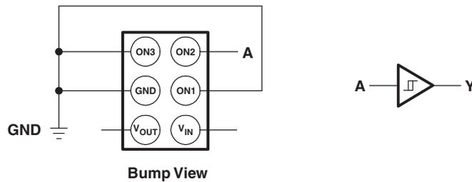
Figure 38. Noninverted Buffer
