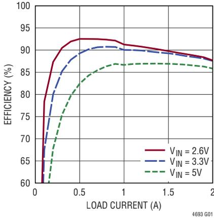
**1.8V<sub>OUT</sub> Efficiency, 1MHz, Burst Mode Operation**
