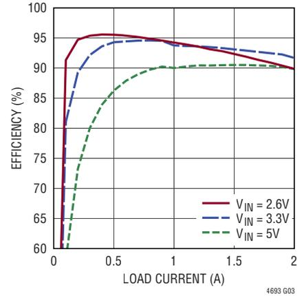
**2.5V<sub>OUT</sub> Efficiency, 1MHz, Burst Mode Operation**
