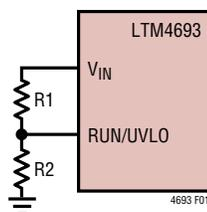
Figure 1. Circuit to Set V<sub>IN</sub> UVLO
