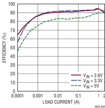
**3.3V<sub>OUT</sub> Efficiency, 1MHz, CCM**
