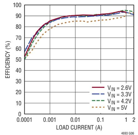
**5V<sub>OUT</sub> Efficiency, 1MHz, CCM**
