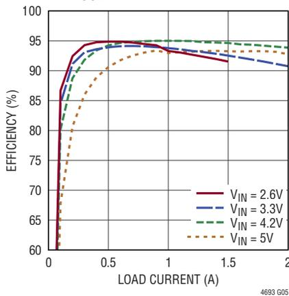
**3.3V<sub>OUT</sub> Efficiency, 1MHz, Burst Mode Operation**
