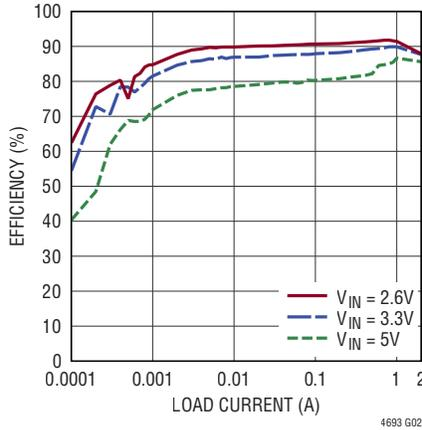
**2.5V<sub>OUT</sub> Efficiency, 1MHz, CCM**
