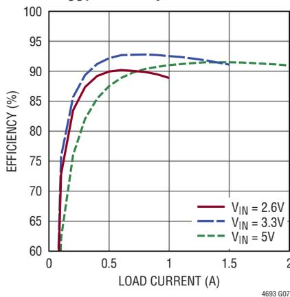
**5V<sub>OUT</sub> Efficiency, 1MHz, Burst Mode Operation**
